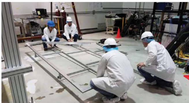
FIG. 2. Exit window frame, with attached support frame.
